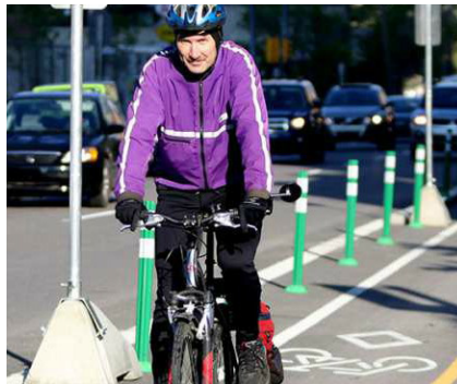
Calgary uses plastic delineators to create an interim design bike lane (City of Calgary).
