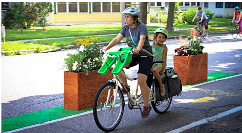
The Minneapolis Bicycle Coalition created 15 plywood planters and set them up to create pop-up protected bicycle lanes at each of the city's summertime Open Streets events. (Kristina Perkins, BikewaysForEveryone. For more information visit: bit.ly/MPLS_StealThisIdea ). Due to their weight, the organization has since created lightweight, collapsible planters that are easier to transport
