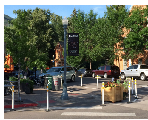
Photos left to right: A Berkeley, CA Protected bikeway demonstration project using cardboard cylinders and a galvanized steel planters (East Bay Bike Coalition - see pages 29 and 39 for more info); A New York City parklet (Street Plans); A pilot curb extension with wooden planters in Aspen, CO (Charlie Simpson); Interim design protected bikeway in Long Beach, CA (Street Plans).
