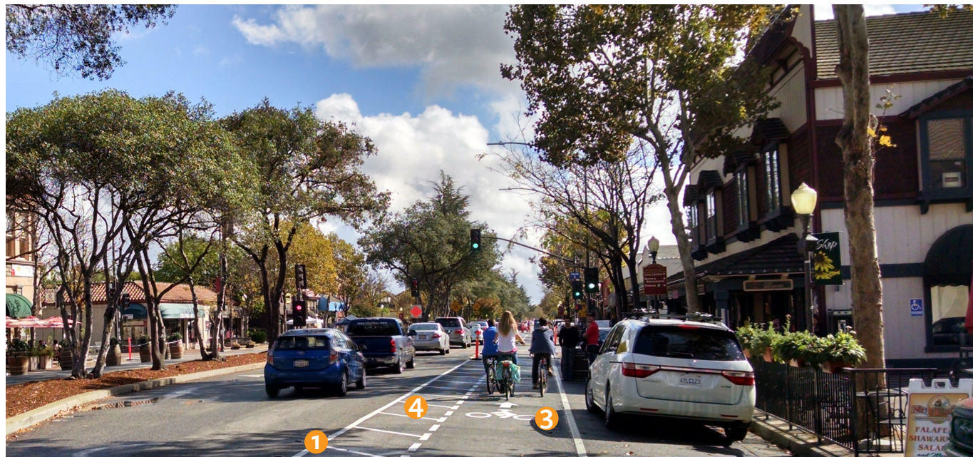
Cheat sheet information based on NACTO Urban Bikeway Design Guide. For more detail, visit: nacto.org . Top: A demonstration planter-protected bike lane in Burlington, VT (Julie Campoli). (Note: For single-lane configurations, this design would require a barrier mountable by emergency service vehicles to be made permanent.) Bottom: A two-day buffered bicycle lane demonstration, Morgan Hill, CA (Street Plans).
